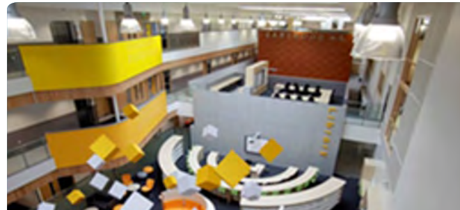
Eastwood High School, Newton Mearns use acoustic cubes to reduce noise
